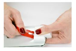
While holding the sensor in place with one hand, pull the red tab to expose the adhesives.
