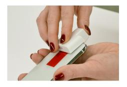
Plug the power connector on the sensor into the device.
