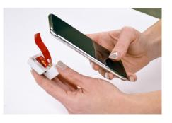
Within the InVue LIVE app, use the camera on your device to scan the code and enroll the sensor. Fill out the information for the sensor and the device that will be displayed.
