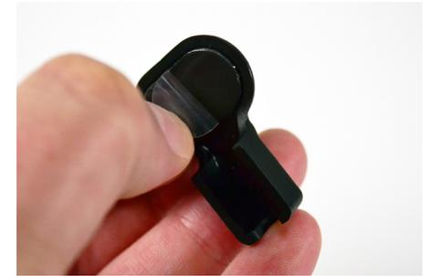
51 Peel the clear film from the 2 adhesives on the power connector protective cap.
