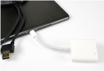
48 Plug the iPad adapter (not supplied by InVue) into the tablet.
