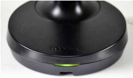
**56** Once a handle is placed on the base, the LED will turn green to indicate that the tablet is receiving power.
