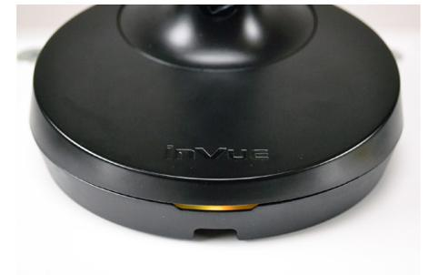
55 If the base is powered up before a handle is docked, the LED on the front will be orange.
