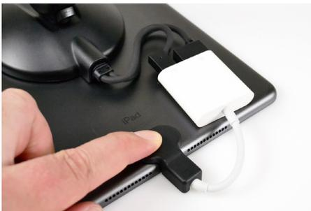
52 Place the protective cap over the power connector, with the adhesives on the back of the tablet. Apply pressure for at least 10 seconds.
