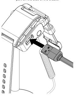
Depending on the wearable and charger type, either remove the wearable from the cradle and place on the charger, or if the charger placement allows, connect the charger to the wearable.
