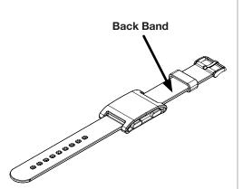
Place the back band of the wearable into the open band clamp with the wearable face down.
