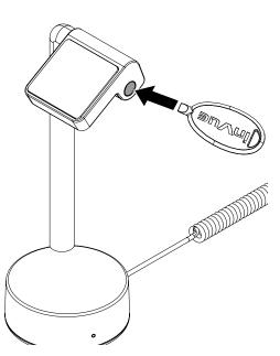
Remove the plug and screw from the side of the cradle.
