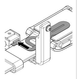
Adjust the wearable so that the area between the 2 white lines on the flex sensor (the shaded area in the below image) will sit over the "hinge" area (the area where the band connects to the watch body) of the wearable.
