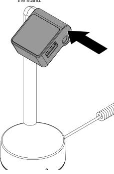
Secure the custom charger cradle with the screw. Insert the plug into the hole in the side on the cradle.
