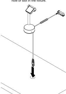
Place the stand in the desired location and apply pressure for at least 10 seconds.
