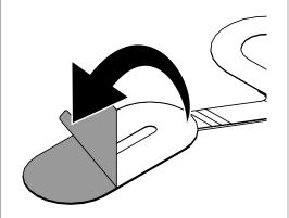
Press the flex adhesive against the bottom of the wearable for at least 10 seconds. Ensure that all of the oval is adhered to the wearable and that no gap is visible.
