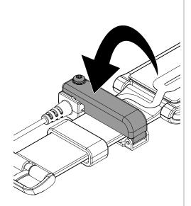
Press down on the band clamp and use a TT8 bit to tighten the screw in the band clamp. Do NOT overtighten.
