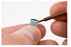
19 Remove the small liner from the adhesive.
