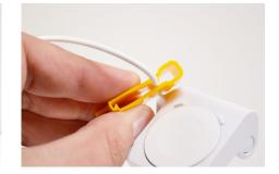
Pull enough cable from the stand to make remerchandising easier. Snap the cable clip over the cable to prevent it from recoiling into the stand.
