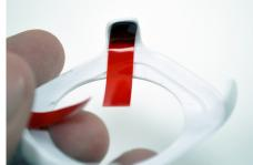
20 Align the adhesive with one of the front corners and smooth it into place for at least 10 seconds.
