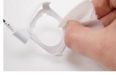
Use a provided alcohol wipe to clean any adhesive residue from the tray sensor. Allow it to dry completely.
