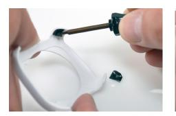
Remove the 2 larger adhesives from the front corners on the tray sensor.
