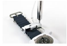
Use a TT8 bit to loosen the screw in the band clamp.
