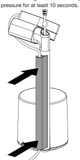
Peel the clear film from the adhesive on the bottom of the stand.
