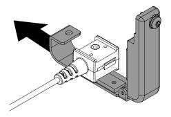
Slide the large band clamp onto the sensor. Proceed with the installation as normal.
