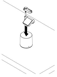
Lift the band clamp from the stand, pulling enough cable to aid in the installation of the wearable. Snap the included cable stop clip around the cable to prevent it from retracting.
