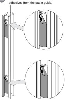
Place the cable guide onto the stem, allow enough room at the bottom for the OEM charger cable to exit. Apply pressure for at least 10 seconds
