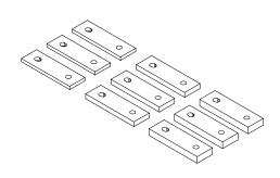
Place the new pad onto the band clamp. Align the holes on the pad with the posts on the band clamp. Apply pressure for at least 10 seconds.
