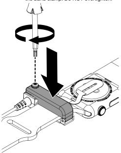
Remove the cable stop clip from the cable.
