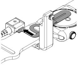
Adjust the wearable so that the area between the 2 white lines on the flex sensor (the shaded area in the below image) will sit over the "hinge" area (the area where the band connects to the watch body) of the wearable.
