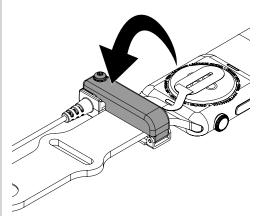
Press down on the band clamp and use a TT8 bit to tighten the screw in the band clamp. Do NOT overtighten.
