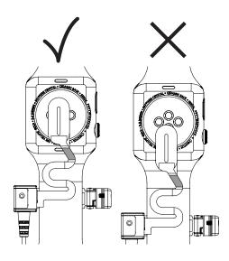
Peel the liner from the adhesive portion of the flex sensor.
