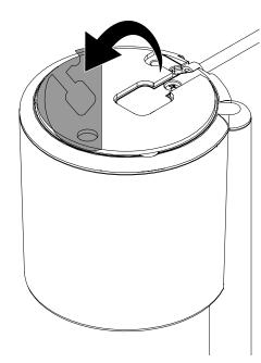
Optional: Route the power cable through a hole or slot in the fixture.
