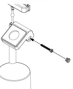
Snap the OEM charger into the trim piece (if applicable). Ensure that the charger is fully inserted and sits flush with the top surface of the trim piece.
