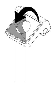
Place the OEM charger/cradle assembly onto the cradle. Make sure that the adhesive sits in the depression and press the trim piece, NOT the charger, against the cradle for at least 10 seconds.
