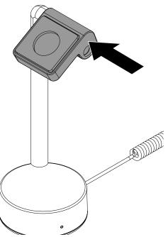
Secure the new cradle with the screw. Insert the plug into the hole in the side on the cradle.
