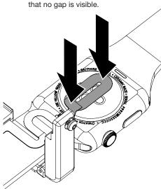
Close the band clamp over the watch band and flex sensor.
