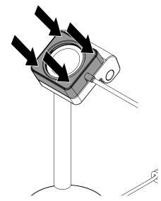
Use the provided alcohol wipe to clean the stem. Allow it to dry completely.
