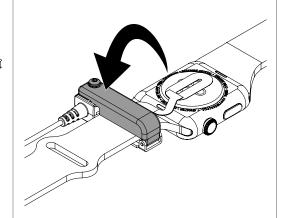
Press down on the band clamp and use a TT8 bit to tighten the screw in the band clamp. Do NOT overtighten.
