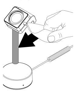
Peel the clear film from the 2 adhesives from the cable guide.
