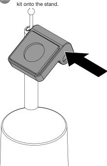
Secure the new cradle with the screw. Insert the plug into the hole in the side on the cradle.
