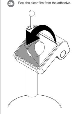
Place the OEM charger/cradle assembly onto the cradle. Make sure that the adhesive sits in the depression and press the trim piece, NOT the charger, against the cradle for at least 10 seconds.
