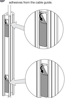
Align the bottom of the cable guide to the top of the base. Apply pressure for at least 10 seconds.
