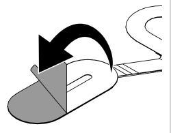
Press the flex adhesive against the bottom of the wearable for at least 10 seconds. Ensure that all of the oval is adhered to the wearable and that no gap is visible.
