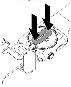
Close the band clamp over the watch band and flex sensor.
