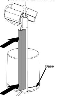
Peel the clear film from the adhesive on the bottom of the stand.
